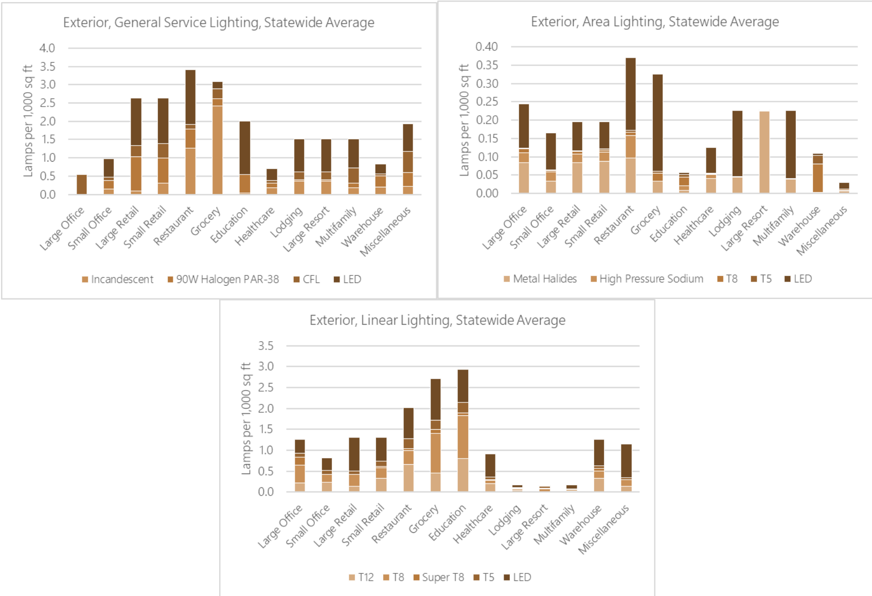
Figure B-8 Commercial Exterior Lighting: Counts of Lamps (per 1,000 sq ft) by Technology and Market Segment
